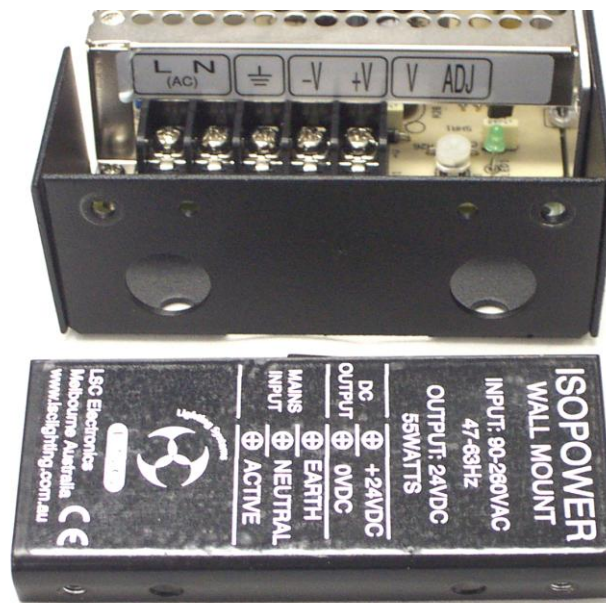
ISPW connections with cover removed
