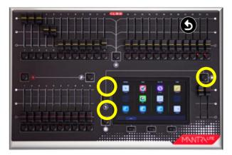
Simultaneously press and hold these three buttons for 0.5 seconds
