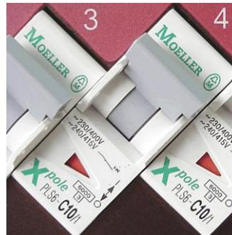
The indicator triangle is green if the circuit breaker has been switched off or has tripped due to a fault.
