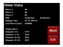
It shows the presence of the input power phases, DMX presence, position of the DMX termination switch, dimmer running time, last cause of a reset and the individual temperatures of the internal modules of the Redback.
