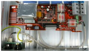
Internal wiring and cable routing. Left hand cover panel removed to show cable routing. Leave in place to avoid damage to static sensitive control electronics.
