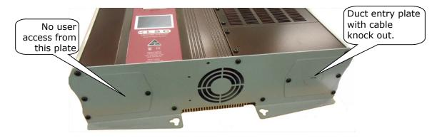
The bottom plate is provided with a cable knock-out entry. To remove the knock-out insert a flat blade screwdriver in the slot provided and twist out the metal disk and fit a M32 cable gland.
